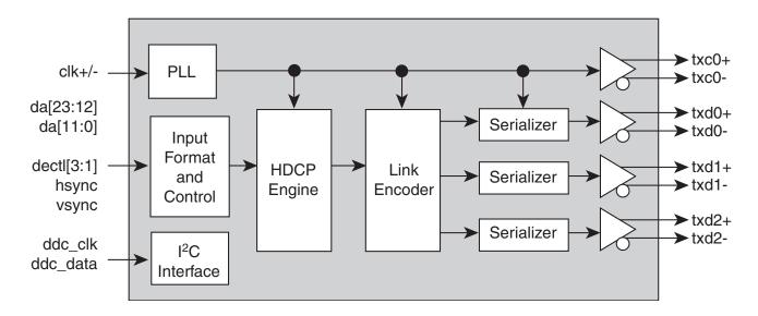
The BCM7501 is part of Broadcom's family of video display products, and is a full rate, single link, DVI 1.0-compliant transmitter with HDCP content protection. The BCM7501 transmits digital video from a digital host such as a PC graphics card, set-top box, or DVD to a display such as an HDTV, flat panel display, or digital CRT. The DVI interface is uncompressed, low-cost, and digitally protected, making it ideal for Consumer Electronics (CE) applications.
